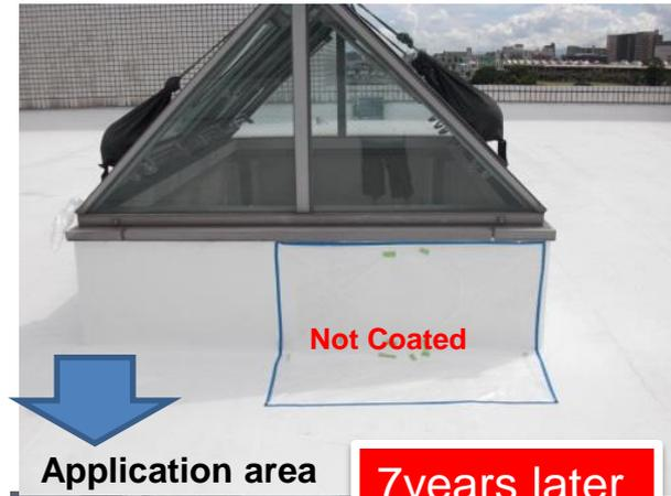
When dirt is really tough like China, Infrared reflectance falls by 5% or more due to dirt., it becomes clean when water is sprayed because the coating surface hard to stick dirt
