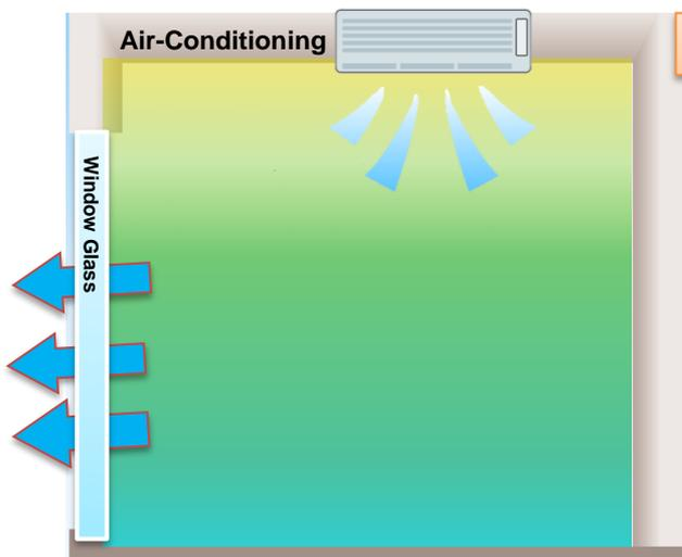
The warm air in the room escapes from the window to the outside and air conditioning efficiency deteriorates.
