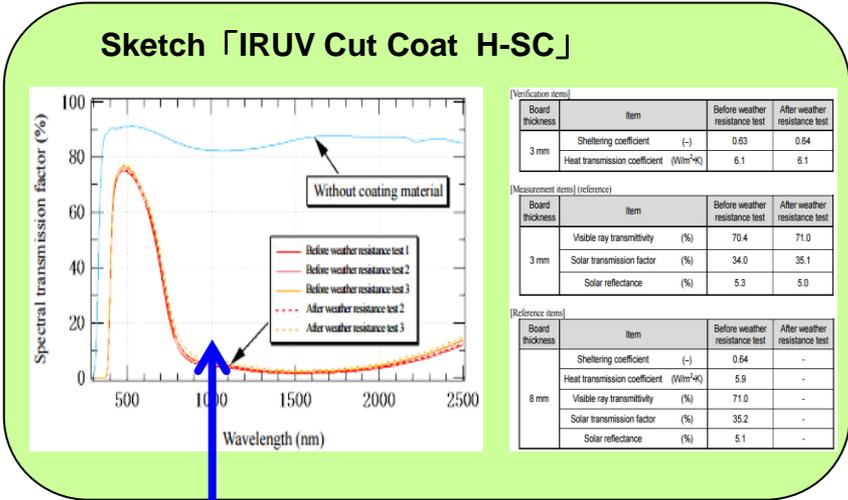
Difference in heat shielding performance in the red part, 2 times performance difference
