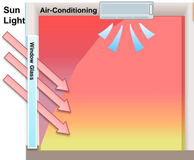
Since the direct heat enters through the window, the room temperature rises and the air conditioner does not work well.
