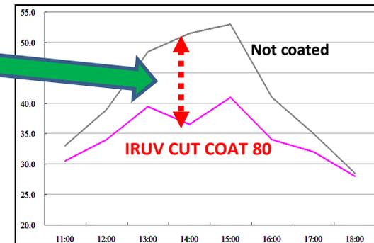
Peak cut from 10 o'clock to 16 o'clock in the daytime is the highest priority for energy saving measures of 'air conditioning'
